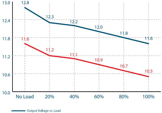
Output Voltage vs. LoadOutput Voltage With a Typical Dimmer
