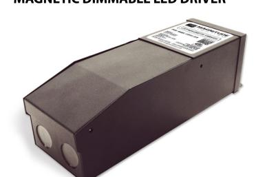
Magnitude's M150L12DC-AR is the most compact LED driver on the market with a magnetic transformer core. It is equipped with two auto-reset breakers, one on the input and one on the output, which protect both the load and driver. The driver is encased in a coated metal box that includes 4 knock-outs, to enable easy installation that complies with electrical code requirements.
